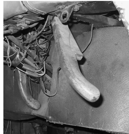
An unusual starting procedure on diesel engined vehicles used a hand brake lever to engage the starter motor. This can be seen in the picture at left.
