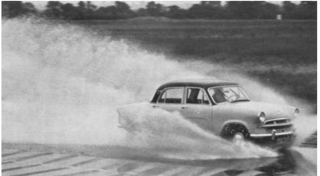
This waterproof test was only one of the many rigorous tests the new Vanguard was subjected to before its release.
