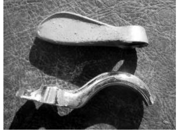
Different quarter vent locks can be clearly seen here with the 1954 curved version at the bottom.
