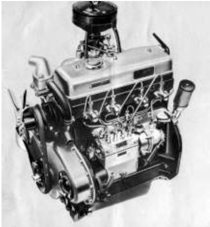
Left. The 2092cc 40 hp Standard diesel engine.
