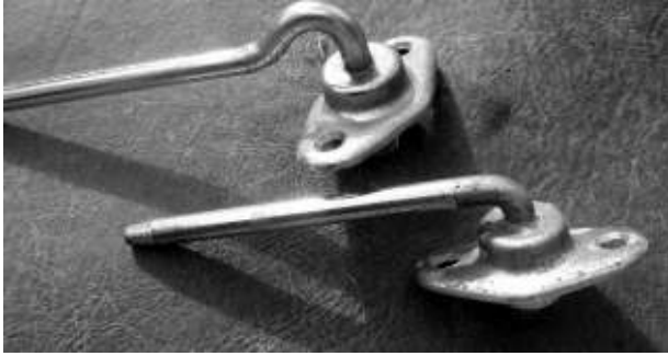
This photo shows the change to the internal sun visor mounting rod .The curved 1954 version is at the top.
