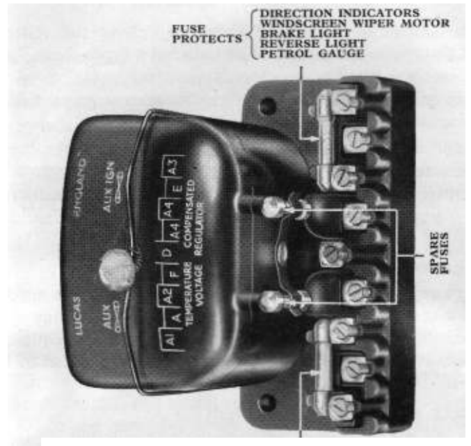
Above - The Combined Regulator/Fuse Box Continued from the 1948 Model
