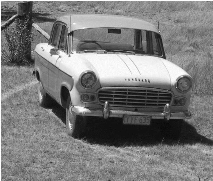
Two chrome strips and the letters V A N G U A R D replaced the star found on previous bonnets.
